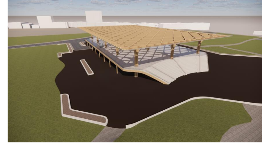
Stage 6 – External Overhang structure (for slandering and draining the roof) is attached to the primary structure.
