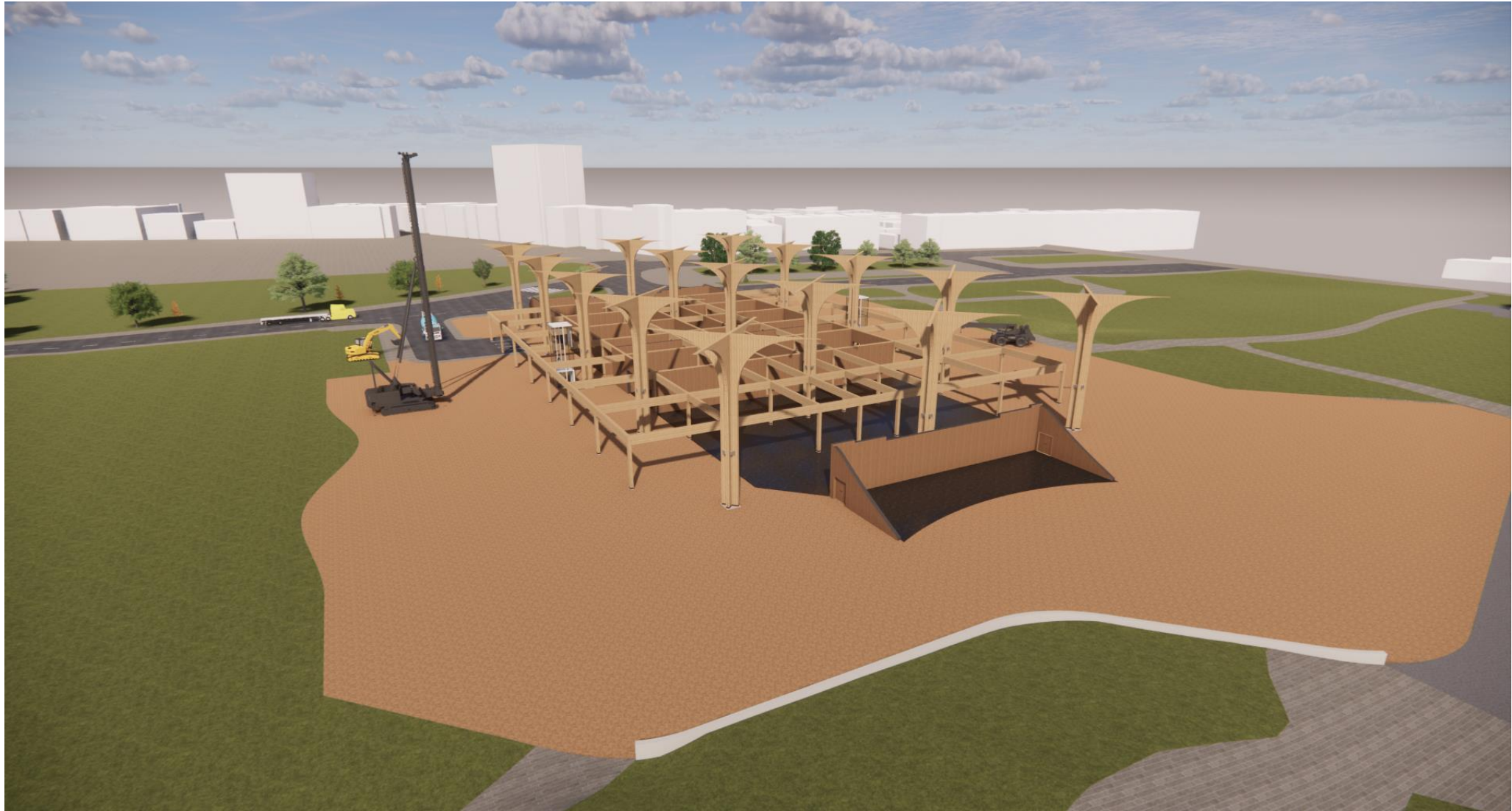
Deck Structure, Canopy Columns, Concrete Base
